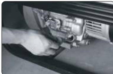
(b) Reinstall the drain plug and fill the engine with oil until it reaches the upper level on the oil filler cap.
